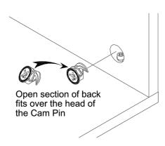
Insert the Cam Lock into the large hole so the opening of the "C" fits over the head of the Cam Pin. You must ensure that the Cam Lock is pushed to the bottom of the hole to catch the top of the Cam Pin.
