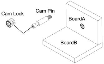
To assemble this product hardware called Cam Lock Fasteners are used. The below is information on how these work.
